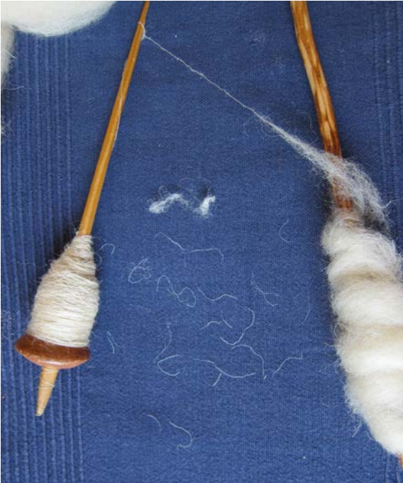
Fig. 9. Spinning wool with kemp, removing the kemp while spinning fine threads (photo: K. GRÖMER).
