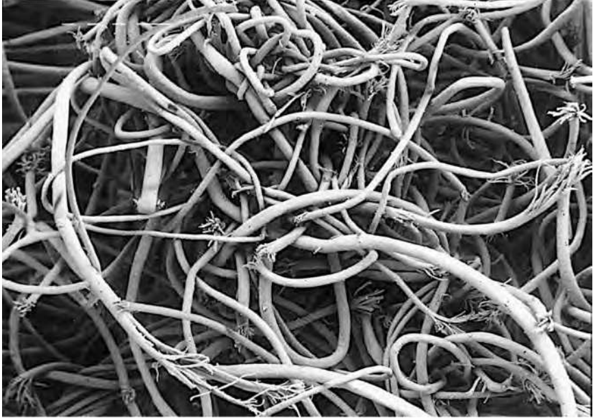
Fig. 3.6. Scanning electron micrograph of a replica of the Vindolanda blanket after 8,000 rubs on a Martindale abrasion instrument. Photo: Lucy Lu, for the Vindolanda Textile Project.
