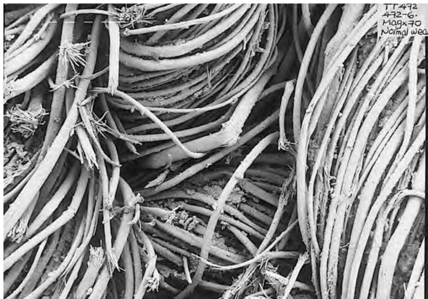
Fig. 3.5. Scanning electron micrograph of a soldier's wool blanket from Vindolanda (VIN88 472) showing 'brush ends' on broken fibres. Photo: Lucy Lu, for the Vindolanda Textile Project.
